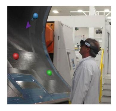
As shown in this picture, the operator can have a very clear view of what type of repairs have to be done on a fuselage panel, as well as how to proceed to this task. Color coded dots show the state of the work to be done, as well as it's precise location thanks to improved anchoring from our identification algorithms.
